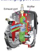
As the piston begins its to upstroke after bottom dead center, burnt gas in the cylinder is pushed out through the exhaust port by lead air. Therefore, almost no air-fuel mixture is emitted.
