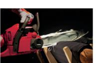
The saw protection consists of a lining with long fibres. If the saw chain cuts through the outer fabric, the fibres get tangled up in the chain.
