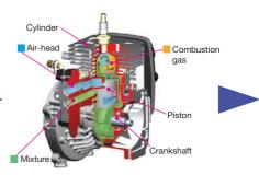
As the piston begins its down stroke after top dead center, a scavenging port starts to open and lead air in the scavenging port moves into the cylinder earlier then the air-fuel mixture
